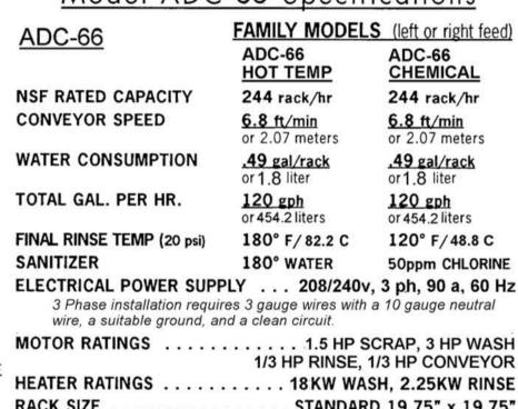
RACK CLEARANCE (Through machine) ..... 19.25" x 20.75"
